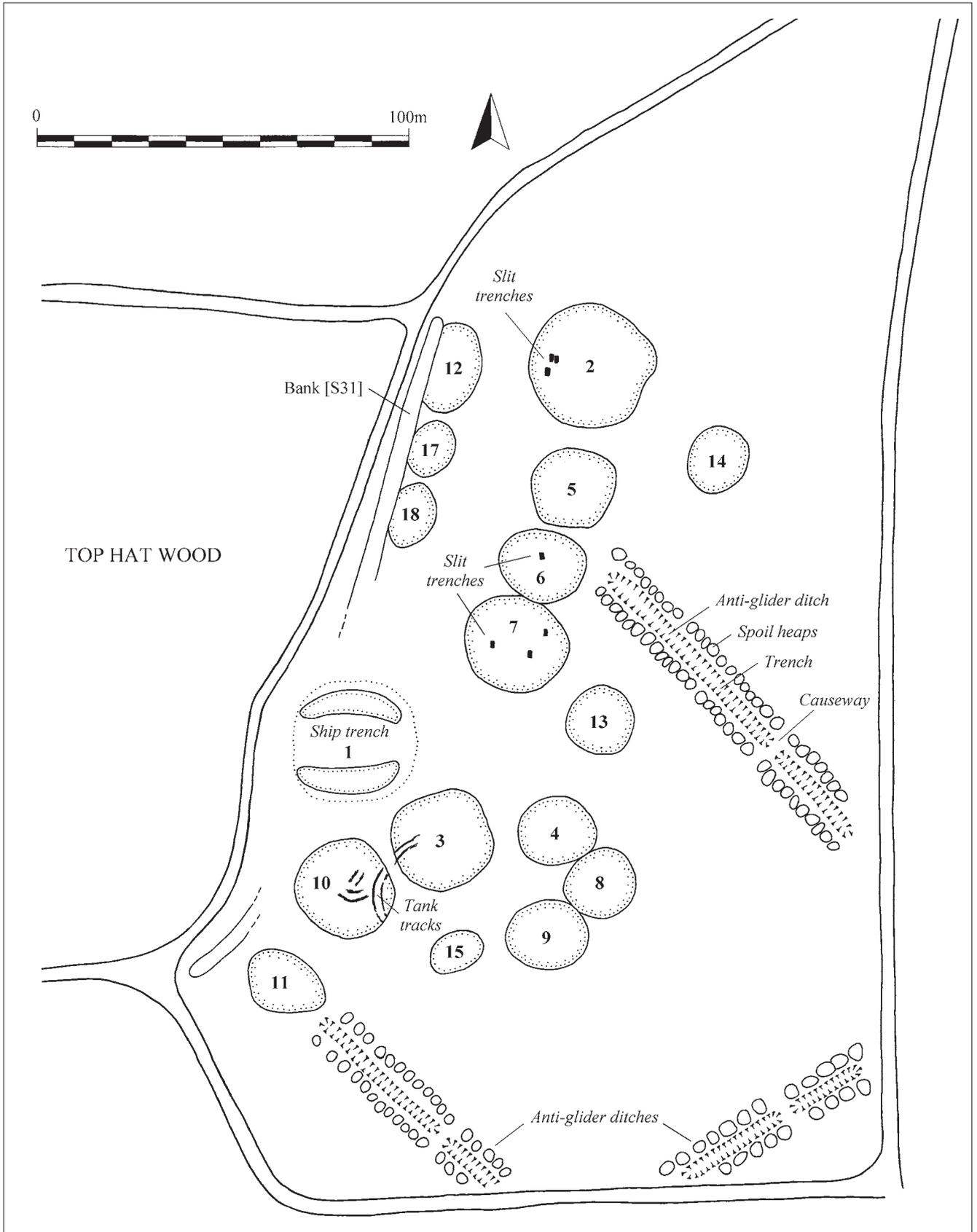
Figure 211 Sutton Hoo at war: plan of anti-glider ditches, slit trenches and tank tracks.
